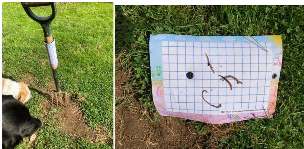
Figure 2: Prototype attaches to the sampling fork so is available for use at any time. The attachment is two stainless steel poppers.
